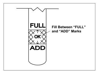
Figure 6. Engine Oil Level
